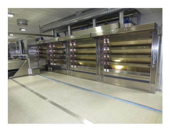
n.4 Tronik deck ovens served by a Robot Loader, with boards pre loading and automatic unloading on accumulation belt
